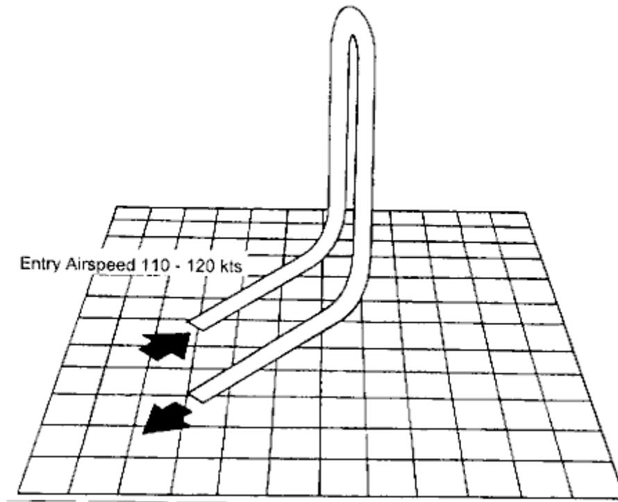
**Figure 16 - Hammer Head Stall Turn**
