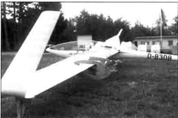
DG-800S of the Akaflieg Karlsruhe used for airfoil drag measurements. A pitot rake is mounted near the midspan point of the left wing. A transducer unit is mounted near the wing root.
