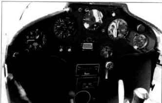
The panel is only just in reach and is far more complex, with a GPS/Data logger and transponder along with the usual array of avionics instruments.
